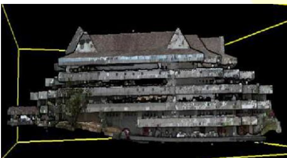
Figure 14 MLS LiDAR Point Cloud of Library
