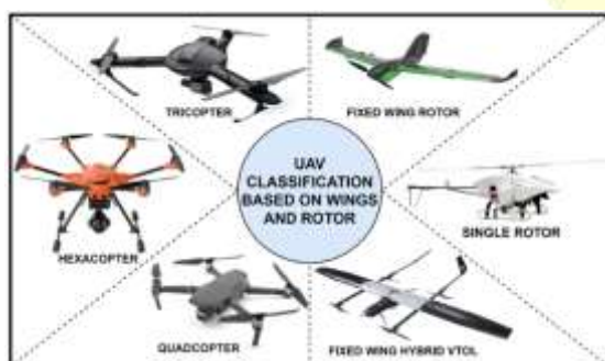
Figure 1 Classification of UAV based on wings and rotors.
