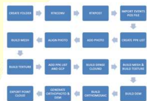
Flowchart 1 Flowchart of image processing from UAV PPK Module
