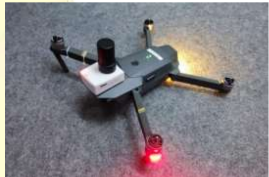
Figure 6 Photo of the DJI Mavic 2 Pro UAV with the PPK Module
