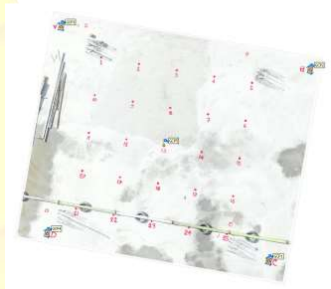
Figure 9 Location of 5 Ground Control Points (GCPs) and 25 monitoring points placed at the Slab Monitoring Area
