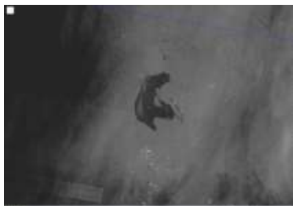
Figure 1. Typical oil spills detected on the Sentinel-1A/1B SAR images: a) large spill around the oil production site (Abouzar oilfield, Iranian sector) on 26.03.2017;
